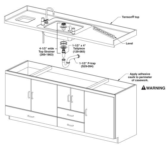
AWARNING The Sink and Deck should be supported properly by casework. The maximum span of unsupported deck should be no greater than 36". If casework does not meet this requirement, add appropriate support such as 1" x 2". Apply silicone caulk to hide seams as needed.
