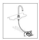
Infrared AC Control Chrome-plated, solid cast brass faucet is available with 10" rigid gooseneck. Electronic faucet is activated when user's hands enter detection area within the lavatory bowl. Flow automatically stops when hands are removed. Flow rate is 1.6 GPM laminar flow.
