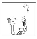
Infrared DC Control Chrome-plated, solid cast brass faucet is available with 10" rigid gooseneck. Battery-operated faucet is activated when user's hands enter detection area within the lavatory bowl. Flow automatically stops when hands are removed. Flow rate is 1.6 GPM laminar flow.
