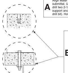
Align water closet waste outlet per rough-in submittal. Using the water closet as a template, drill two 2-1/8" deep holes into the water closet support anchoring locations (use a 5/8" concrete drill bit). Holes must be clean and free of debris.
