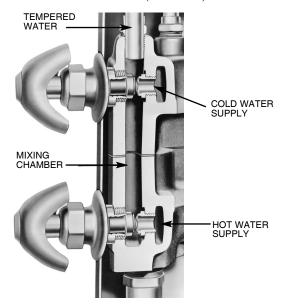
The hot supply to these valves should always be tempered by a master controller, either at a remote location or mounted in the shower equipment.
