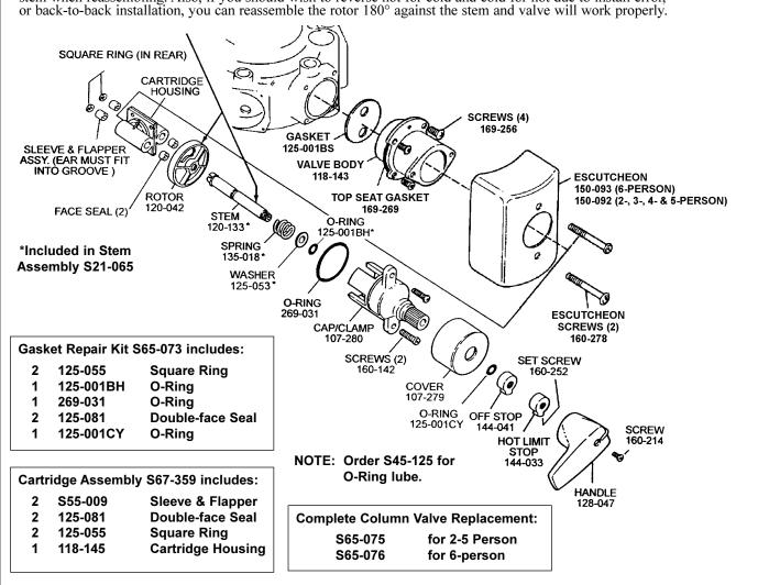
Valves are equipped with a temperature limit stop which can be used to limit the temperature of tempered water discharged. To adjust the temperature, remove the handle and loosen the set screw. Remove the limit stop and reposition to desired setting. Turn the limit stop clockwise for a hotter setting and counterclockwise for a cooler setting.
