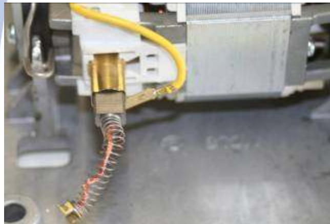
Step 1: Press the clip which is covering the brushes.
