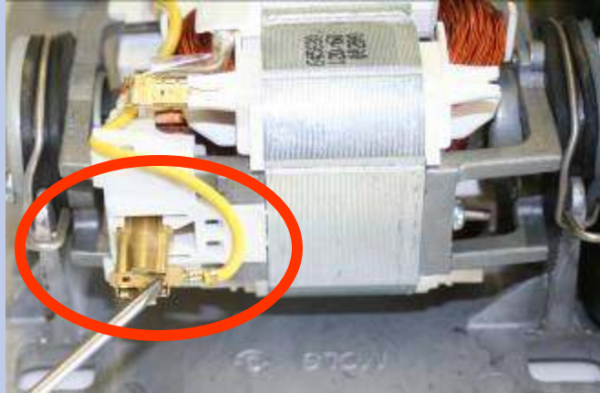
Step 1: Press the clip which is covering the brushes.
