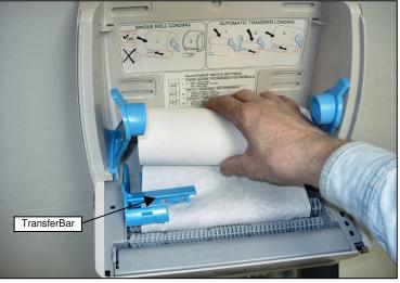
2) Carefully remove the stub roll, making sure the paper web is under the transfer bar.
