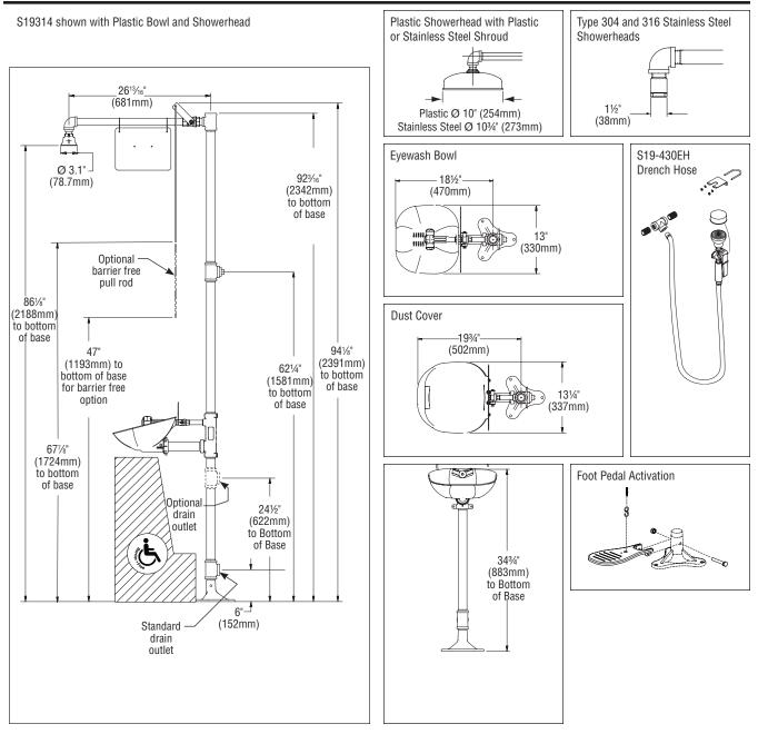
All dimensions assume standard thread engagement. Variations in manufacturing allow for  $+/-\frac{1}{6}$ "(3mm) per threaded joint. To find the tolerance of a dimension, add the number of thread joints across the length of the dimension and multiply it by  $\frac{1}{6}$ " (3mm).
