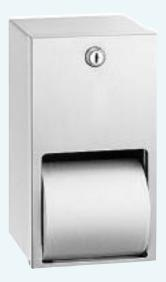
**Best:** Heavy traffic applications require a jumbo roll toilet tissue unit, such as this unit, which holds two large 9-inch individually dispensed rolls. Using very large rolls means less servicing. A bottom hinged front panel is secured with a tumbler lock to prevent vandalism and theft.
