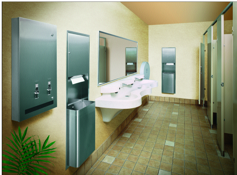
Group handwashing stations have fewer plumbing connections than traditional lavs, and a tankless water heater can be concealed within a pedestal. Rather than heating an entire water tank, these fixtures only heat the water needed at the faucet.
