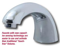
technology creates an omni-directional detection zone that surrounds the entire spout, rather than a sensor window commonly used with infrared-controlled faucets. All of the faucet's mechanical and electrical components are concealed in a water-resistant housing.
