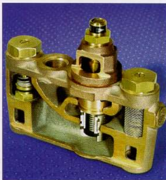
A cross-section of a thermostatic mixing valve shows where the hot and cold water are blended to produce tempered water.
