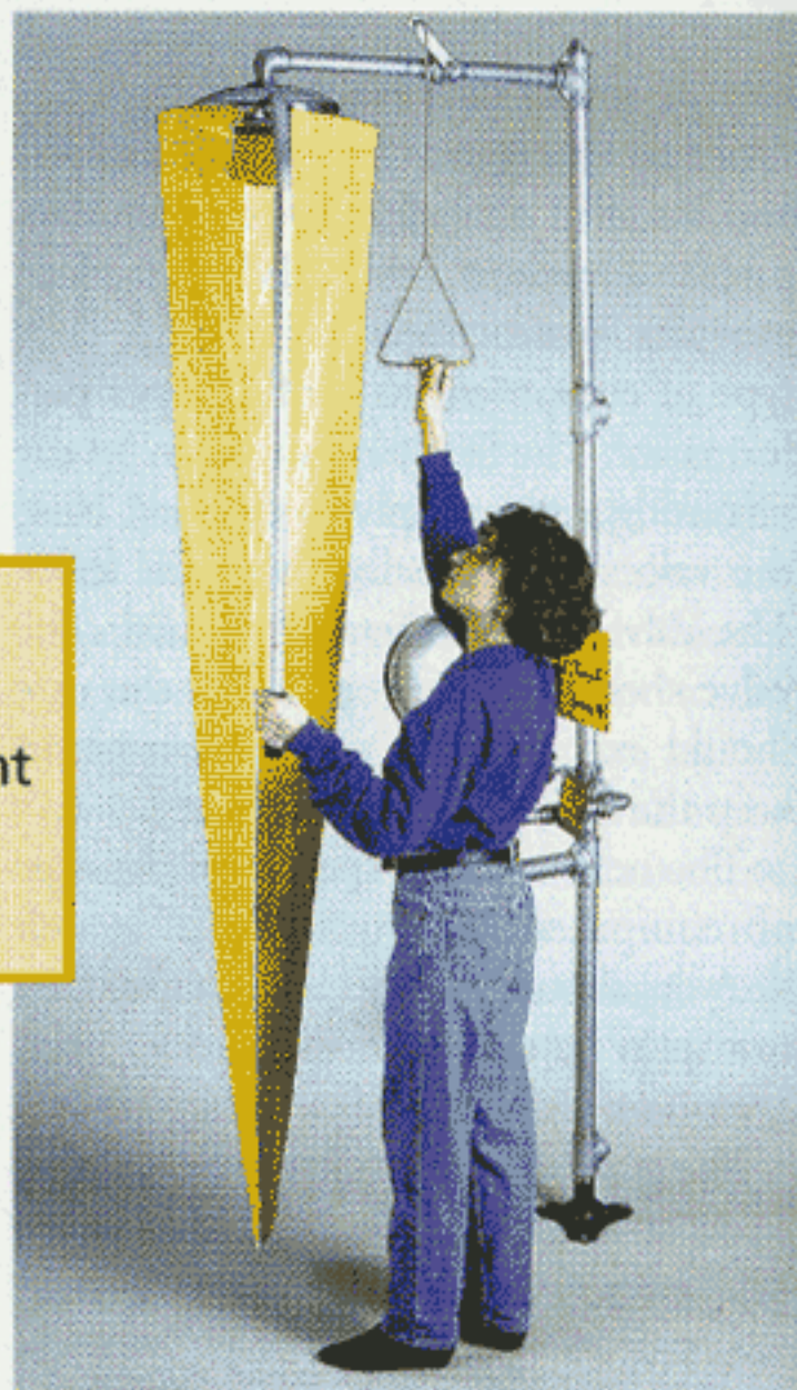
Tester provides a way of testing drench showers to comply with ANSI specifications for weekly testing without getting wet. The watertight funnel has a weighted bottom and directs water to a drain or bucket.
