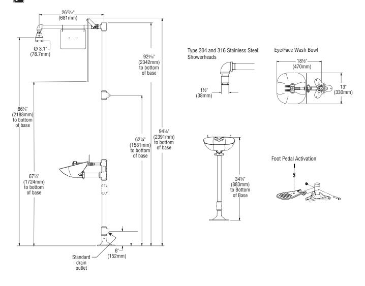
All dimensions assume standard thread engagement. Variations in manufacturing allow for +/- ½"(3mm) per threaded joint. To find the tolerance of a dimension, add the number of thread joints across the length of the dimension and multiply it by ½" (3mm).
