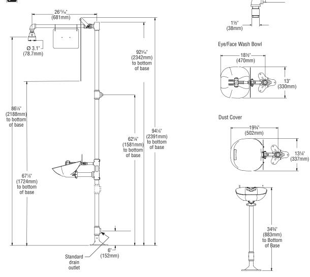
All dimensions assume standard thread engagement. Variations in manufacturing allow for +/- ½"(3mm) per threaded joint. To find the tolerance of a dimension, add the number of thread joints across the length of the dimension and multiply it by ½" (3mm).
