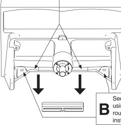
Secure the bowl to the wall anchors using fasteners per the structural rough-in requirement (supplied by installer).
