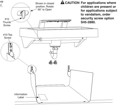
Rotate access panel up and secure by rotating thumbscrews to the closed position
