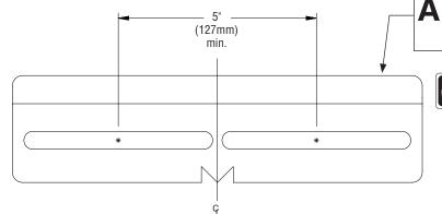
Install wall bracket to wall per structural rough-in dimensions. Check to ensure the bracket is level. Example anchor locations shown.
