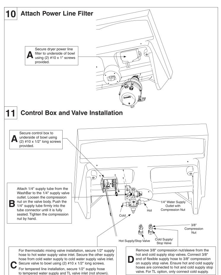
Secure valve to bowl using (2) #10 x 1/2" long screws.
