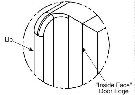
**B** With the door in the closed position, place the strike/keeper on the pilaster so the top edge is 1/4" (6mm) above the bottom of the latch slide bar and the leading edge is lined up with the edge of the pilaster notch (approximately 5/8" [16mm] from the side of the pilaster). Using the strike/keeper as a template, mark the hole locations and drill  $\varnothing 7/32$ " pilot holes, 3/4" (19mm) deep. Secure the strike/keeper to the pilaster with the #14 x 3/4" screws provided.
