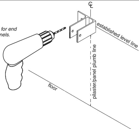
**A** Place the center of each stirrup bracket at the established level line. Center the bracket opening on the pilaster/panel plumb line.
