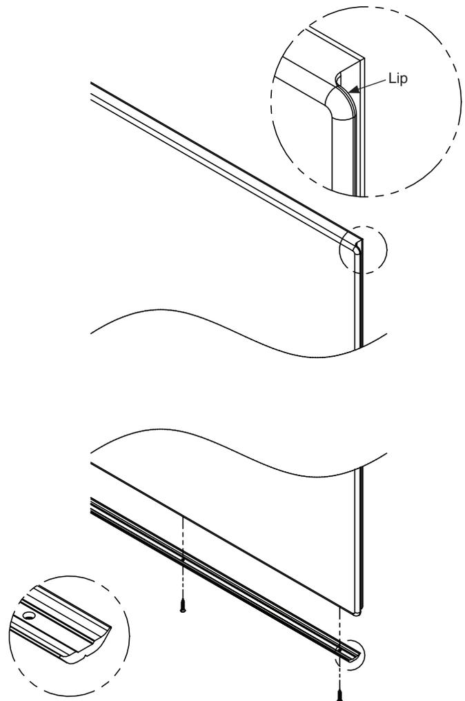
**9b Continuous Spring-Loaded Piano Hinge - Stainless Steel (Optional)**
