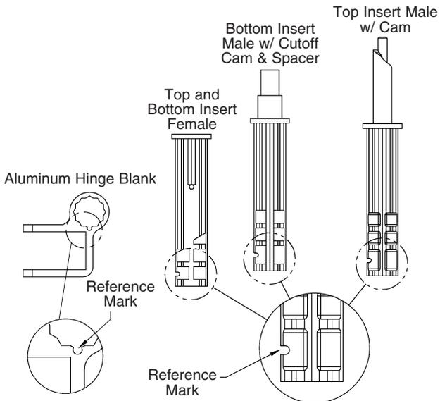
**B** Find the hinge assembly that coincides with the door swing. Arrange the hinge sets as shown.
