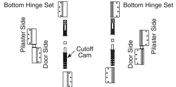
**D** Assemble inserts into the hinge blanks making sure the insert collar fits tightly against each of the hinge blanks.
