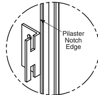
**D** Position the coat hook 36" (914mm) above finished floor (hook goes on the inside of compartment). Using the hook as a template, drill (2)  $\varnothing 7/32$ " pilot holes, 3/4" (19mm) deep. Secure with the #14 x 3/4" screws provided.
