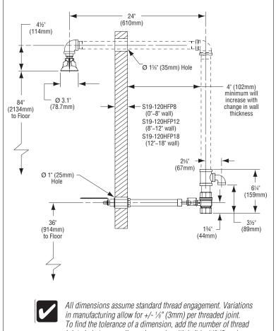
joints in between a dimension and multiply it by 1/8" (3mm).
