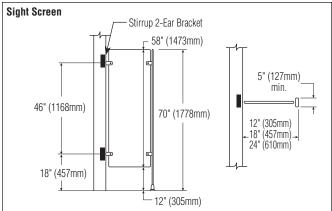
Generally recommended for Sight Screen application. Screen has floor mounting and requires minimum 3" concrete floor for anchoring.
