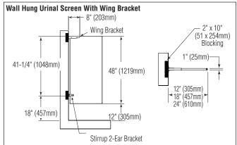
Generally used for Urinal Screen application where added durability is needed for high traffic areas. Screen is mounted to wall with Mills chrome plated wing bracket and 2-ear stirrup bracket.
